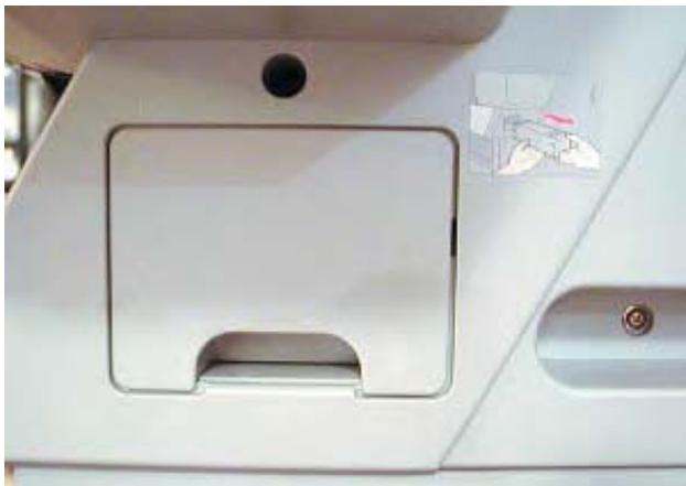
Another item that is chipped is the “maintenance tank. The purpose of this tank, located on the right side of the printer just above the stand is to collect ink purged from the printhead during either cleaning, cartridge replacement, or cartridge removal (when the printer is to be moved
