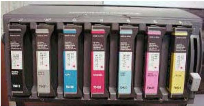
tion of inkset being made when the original ink cartridges, the ones that came with the printer, are inserted. These cartridges have special chips which tell the printer whether it will be a dye or a pigment printer.
